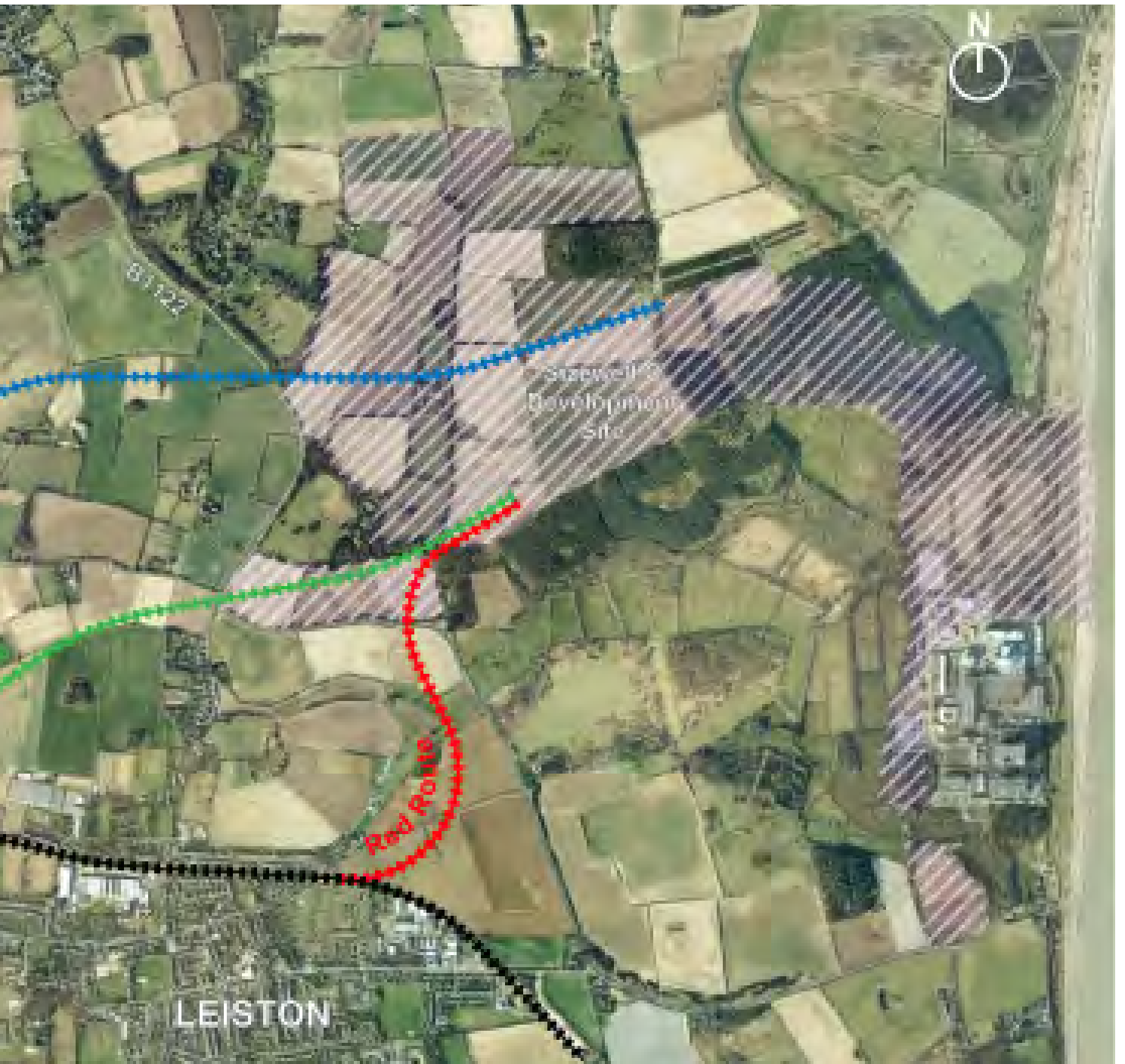
Figure 6.17: Potential route options for rail line extension (Option 2)
