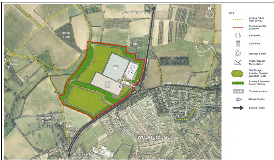
Figure 5.4.7: Park and Ride South Option 2 – Schematic Zoning Diagram
