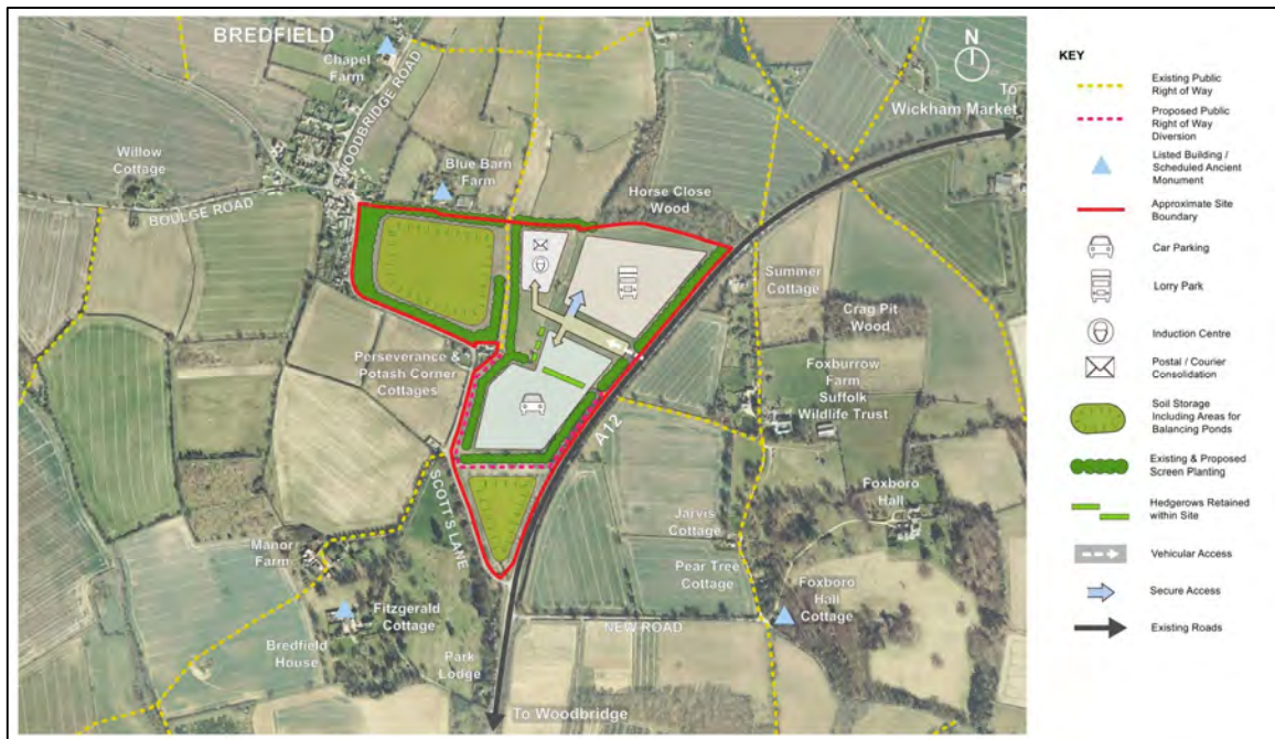
Figure 5.4.8: Park and Ride South Option 3 – Schematic Zoning Diagram
