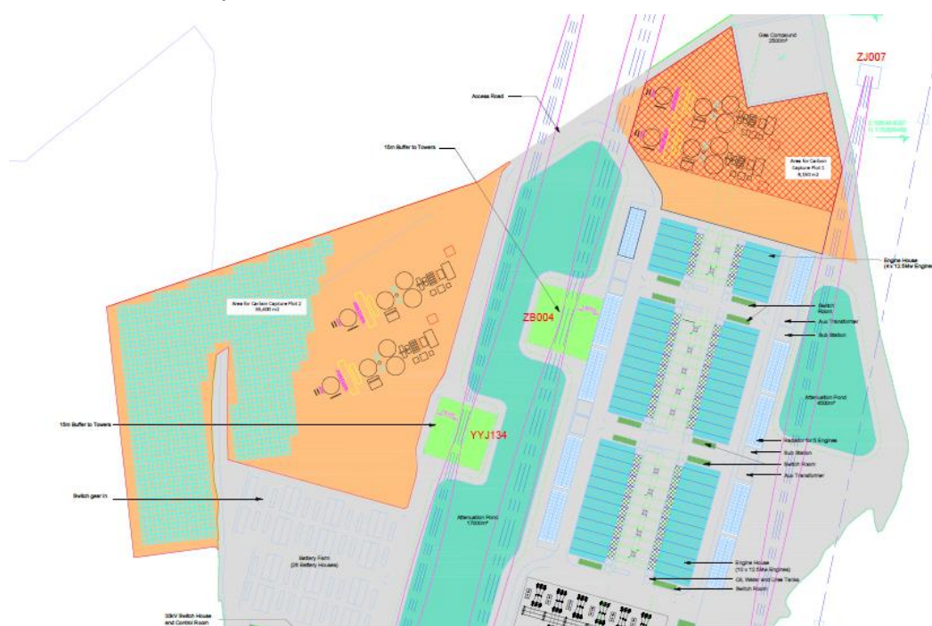
Figure 4: Indicative carbon capture layout
