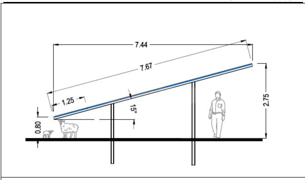
Illustration 4.3: Array of Ground Mounted Solar Panels - Cross Section Detail
