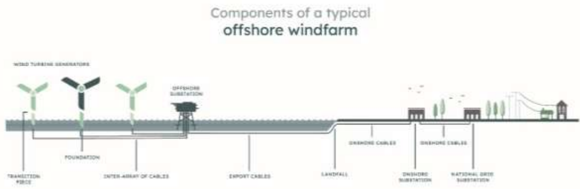
Figure 2: Components of a typical offshore wind farm
