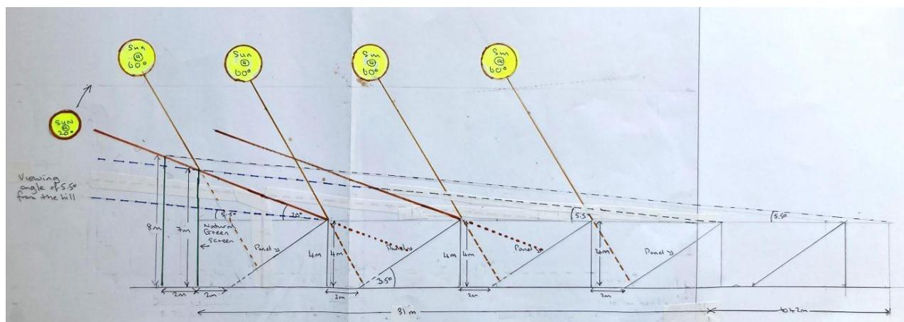
Evidence is available, with calculations, in Appendix 1, which shows that locally the sun barely generates any power at angles less than 20°. Even at this angle the drawing shows that a large area of all panels behind the front row will be screened by the panels in front of them. i.e. the applicant's design includes a high level of screening which would prevent power generation even when the sun is less than 20°.
