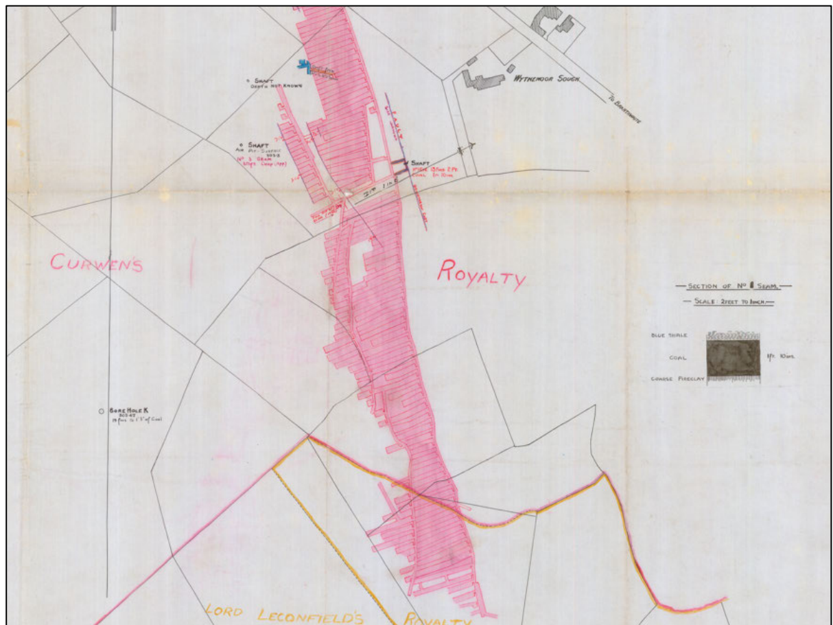
Figure 3.1: Extract of mineplan showing extents of workings at the level of the No.1 Coal. 8
