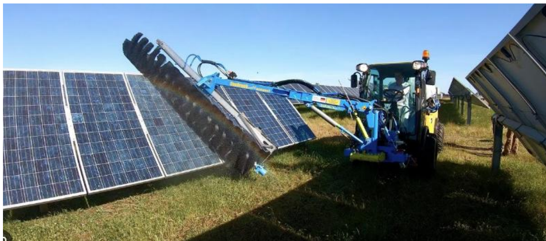
Photo 17.43: Cleaning of Solar Modules
