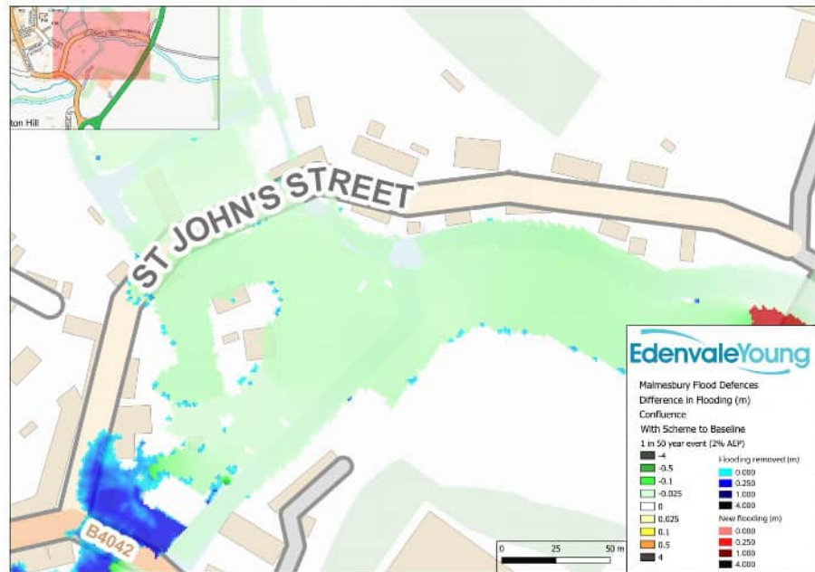
Figure 7.9: Peak Level Difference Map for 1 in 41 year return period flood event local to the Sherston/Tetbury Avon confluence
