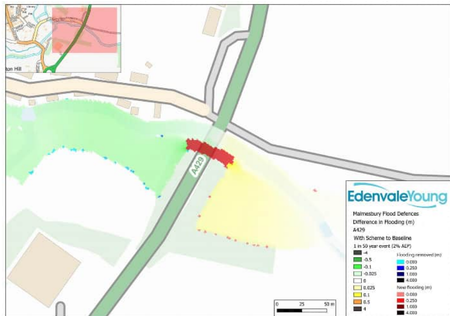
Figure 7.14: Peak Level Difference Map for 1 in 41 year return period flood event local to the A429 road bridge
