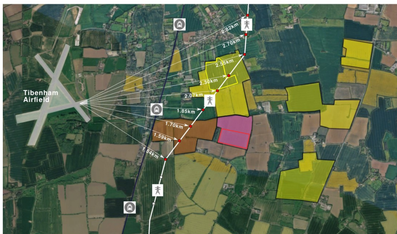
Figure 3: Pylon Distances from Take-Off Point Runway 08
