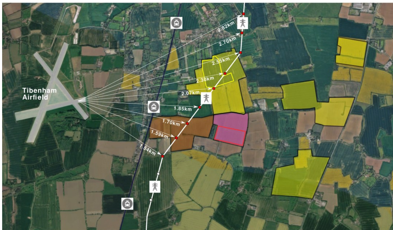
Figure 1: Pylon Distances from Take-Off Point Runway 08
