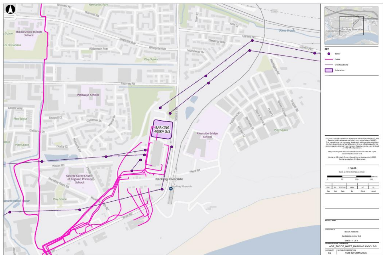
Figure 2: NGET Assets in proposed development area (BARKING 400KV S/S)
