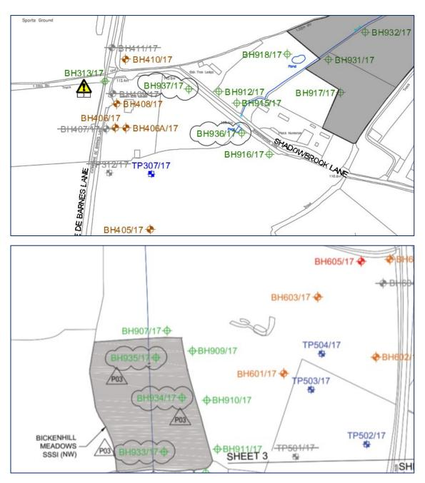
Figure 11A (top) and 11B (bottom) Ground Investigation locations – extended to include the SSSI units. Red – cable percussion boreholes; orange – rotary coring boreholes; green – window sample; blue – trial pit.
