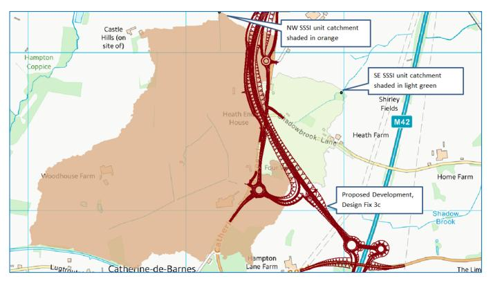
Figure 8. Catchment boundaries as determined from GIS catchment analysis, with the Design Fix 3C road alignment overlain in red.
