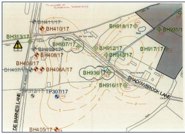
Figure 13A (top) Contours showing top of the Mercia Mudstone (m AOD) and 13B (bottom) Contours showing thickness of superficial deposits (m). Plots are based on available information (November 2018).
