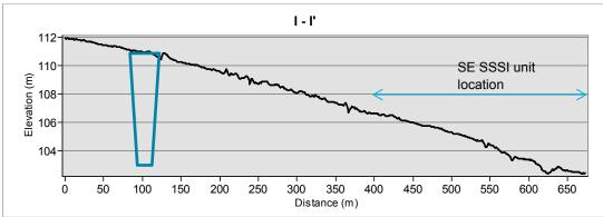
Note. Indicative cutting of up to 8m depth shown in blue in this topographic section.
