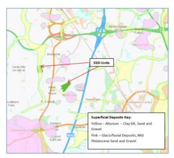
Figure 5. Superficial deposits in the area around Bickenhill Meadows SSSI (source: British Geological Survey Geoindex website, http://www.bgs.ac.uk/geoindex).
