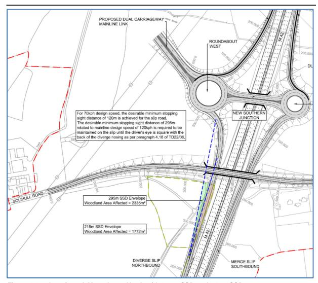
Figure 3.2 – Junction 5A Moved 50m North with 295m SSD and 215m SSD
