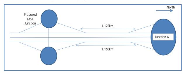
Figure 2 – Proposed MSA Junction and Weaving Lengths on M42 Motorway (Derived from Stage 2 technical Note based on MSA Planning Application Documents)
