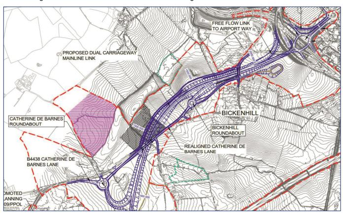
Figure 7. Contour map to show topography surrounding the two SSSI units. SSSI units are outlined in a green dashed line, with the Scheme red line boundary shown in red). Contours were derived from topographic survey undertaken at PCF Stage 2 for the Scheme.
