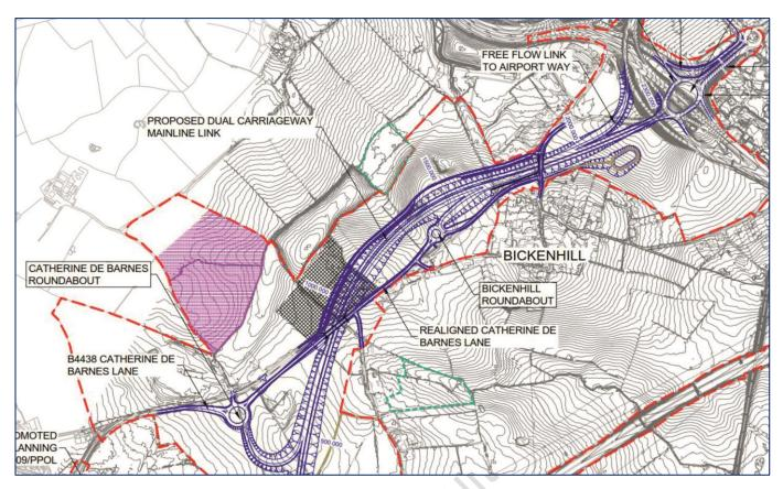
Figure 7. Contour map to show topography surrounding the two SSSI units. SSSI units are outlined in a green dashed line, with the Scheme red line boundary shown in red (which has since been modified). Contours were derived from topographic survey undertaken at PCF Stage 2 for the Scheme.
