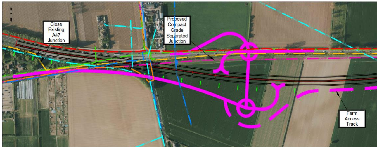
Figure 4-3: Yarmouth Road Junction arrangement, Option C
