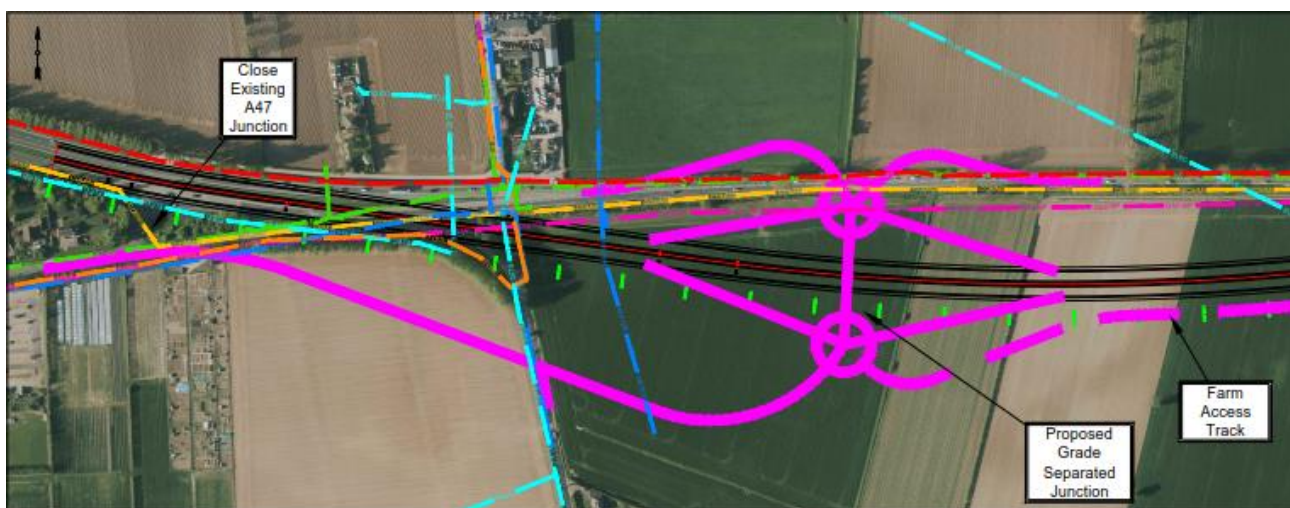
Figure 4-2: Yarmouth Road Junction arrangement, Option B
