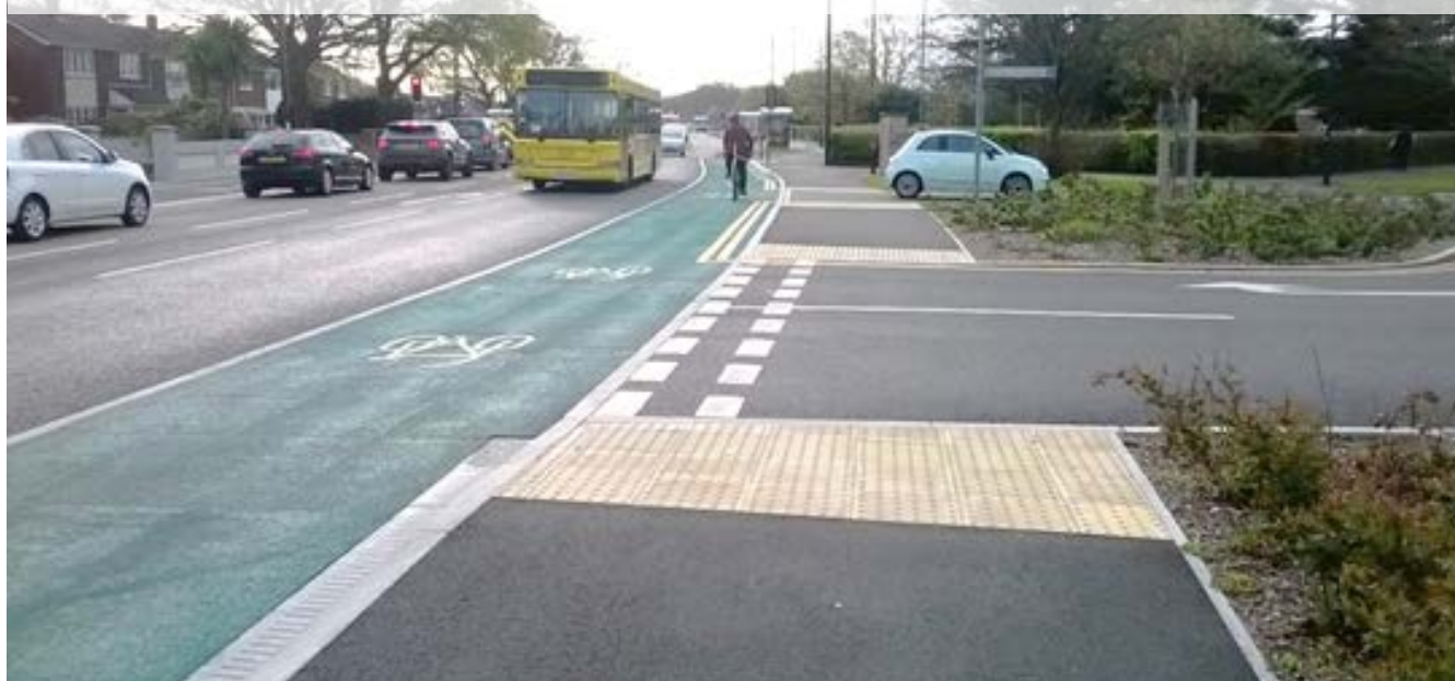
Figure 10.17: No setback crossing with design priority, – Bournemouth
