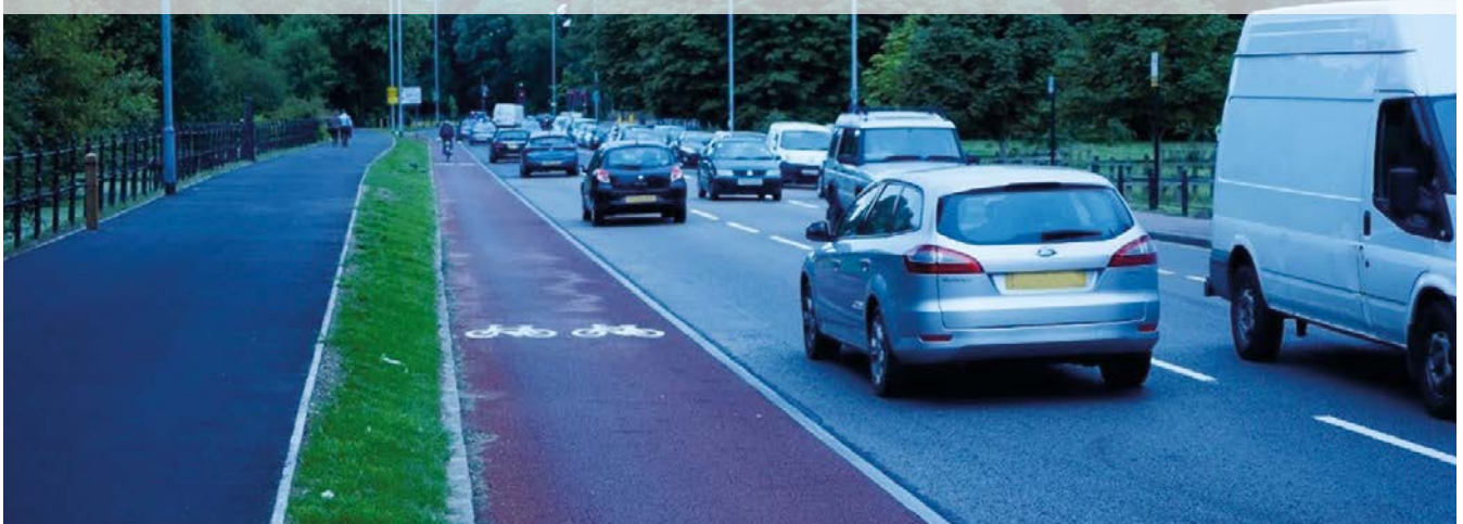
Figure 6.13: Double TSRGD diagram 1057 symbols on one way stepped cycle track, Cambridge
