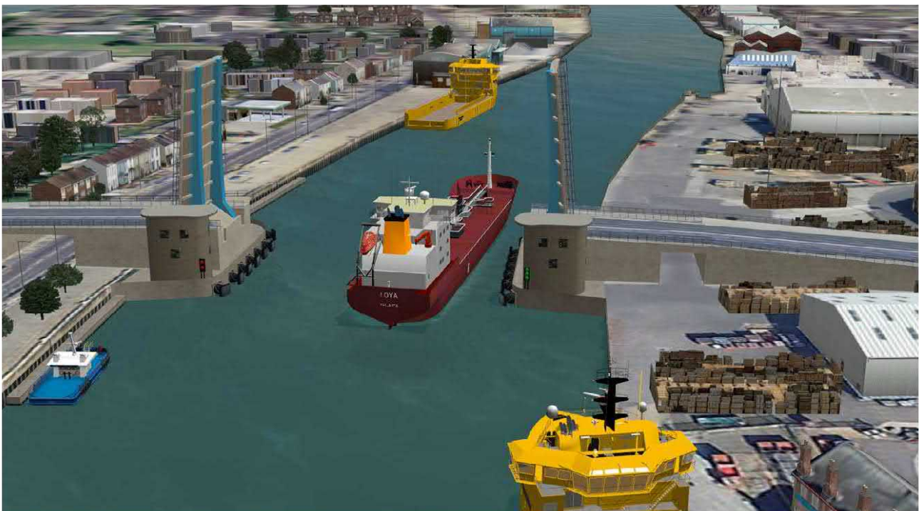
Figure 8.50: Run 24: 4m minimum clearance to east knuckle
