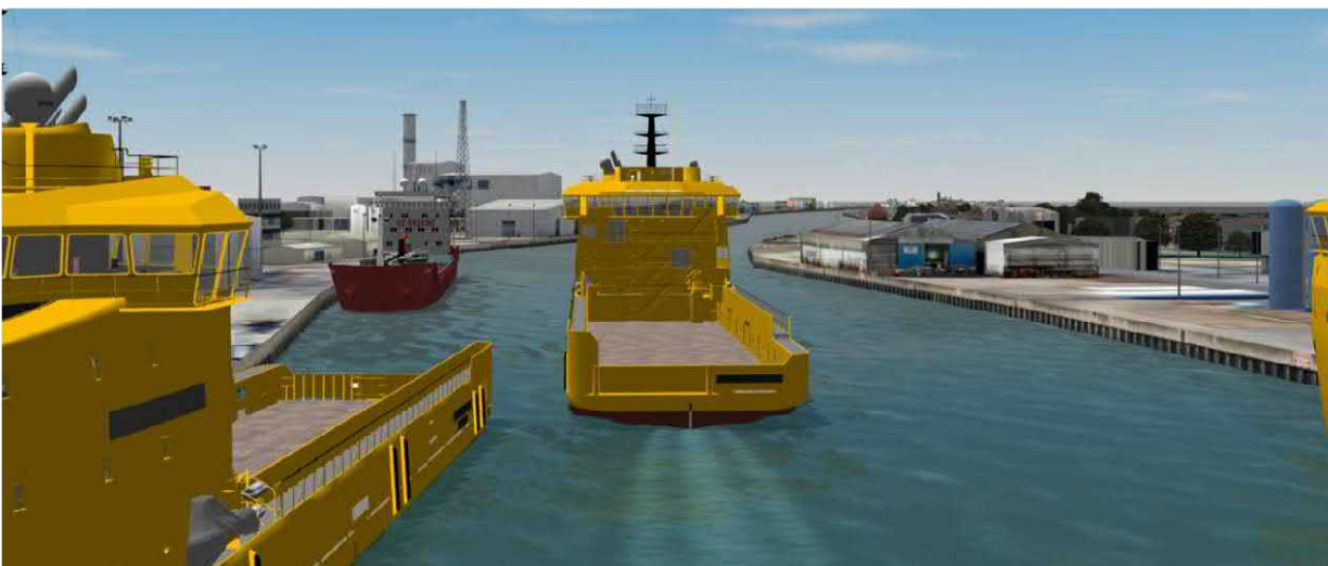
Figure 8.32: Run 07: Outbound PSV passing close to moored PSV, 06 minutes elapsed
