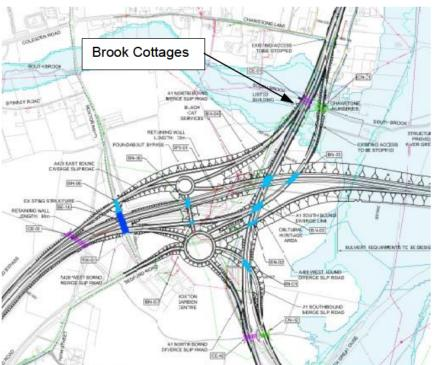
**Option A** – Option A consisted of a three-tier grade separated junction with a dumbbell roundabout located between Roxton Road and the existing Black Cat roundabout. This option required removal of Brook Cottages.
