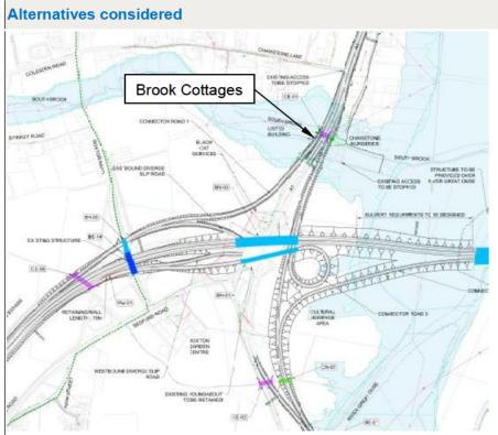
**Option B** – Option B involved the construction of three main connector roads in the vicinity of the A428 and the A1 based on the most significant traffic flows. This option required removal of Brook Cottages.
