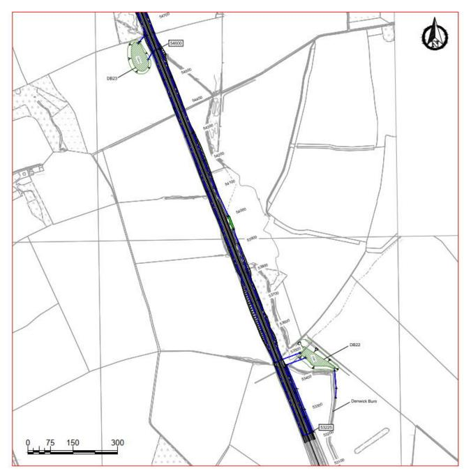
Figure 4-1 - Highway Drainage Layout and Detention Basin DB22 PRELIMINARY DESIGN STRATEGY:
