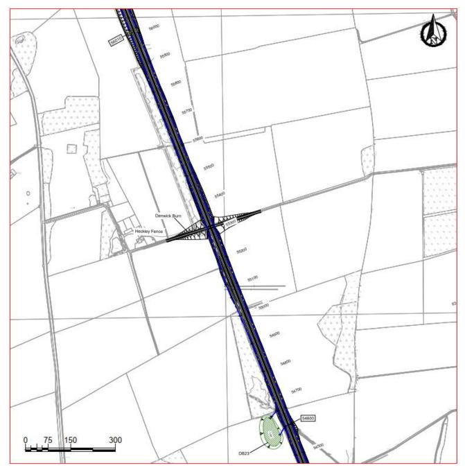
Figure 4-2 - Highway Drainage Layout and Detention Basin DB23 PRELIMINARY DESIGN STRATEGY:
