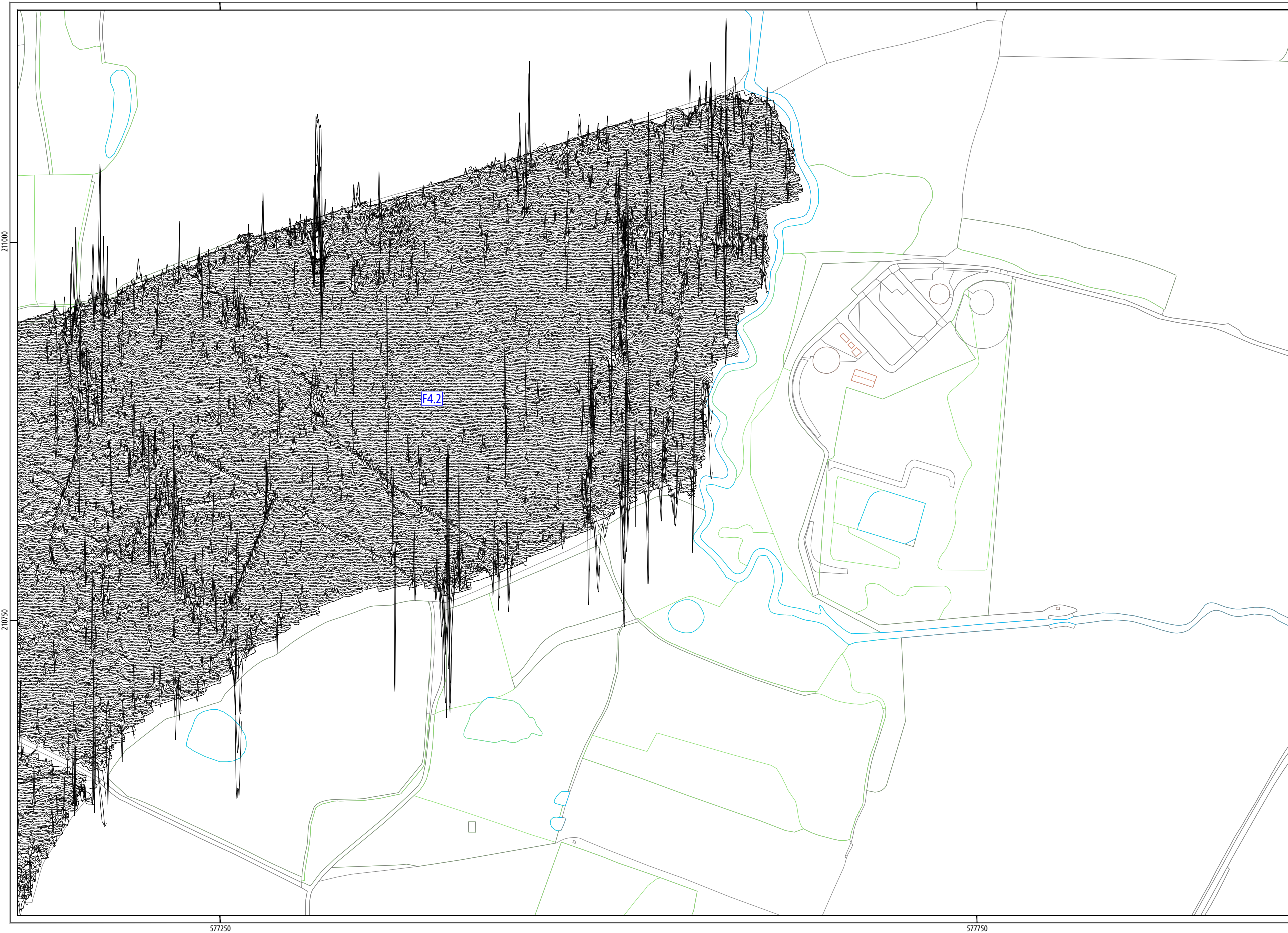
ILLUS 23 XY trace plot of minimally processed magnetometer data; Sector 5
