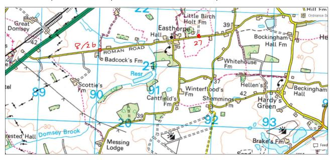
In the June 2021 consultation, the historic and current, albeit now access limited connection, between Easthorpe Road and the A12 was retained with a new vehicular bridge taking Easthorpe Road over the new A12 and Easthorpe Road continuing onto a junction on the (de-trunked) A12.
