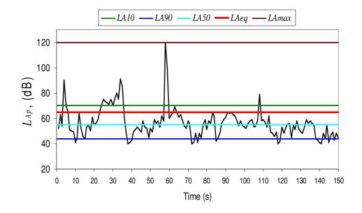
SPL, LpSound pressure level - The level of sound pressure;<br/>expressed in decibels, as measured by a standard sound<br/>level meter with a microphone. This differs from Lw in<br/>that this is the received sound as opposed to the sound<br/>'intensity':
