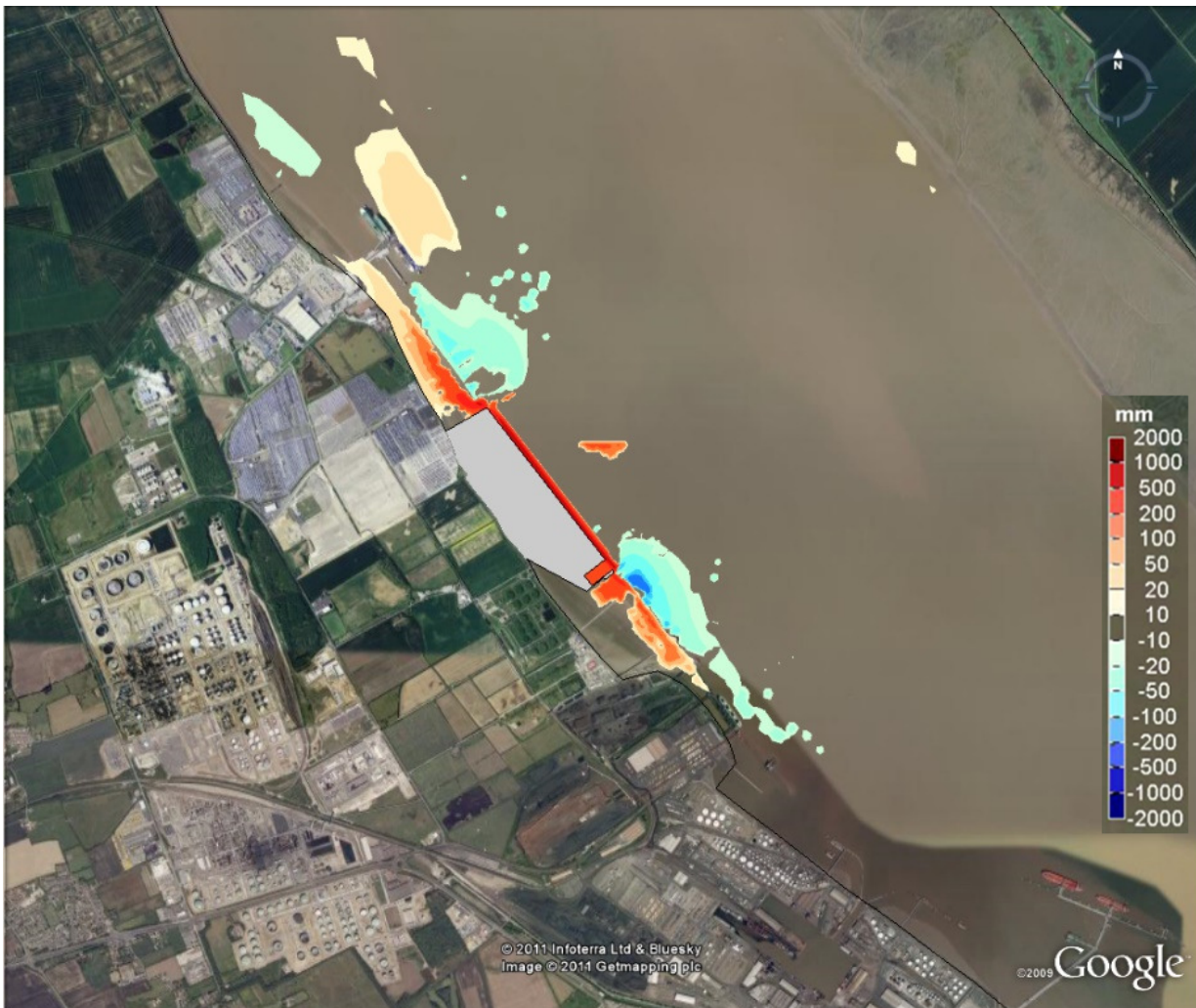
Figure 8-36: Predicted increases to deposition or erosion of muddy sediments after a spring-neap cycle (AMEP minus baseline (consented)). From Annex 8.3 (HR Wallingford, 2011)
